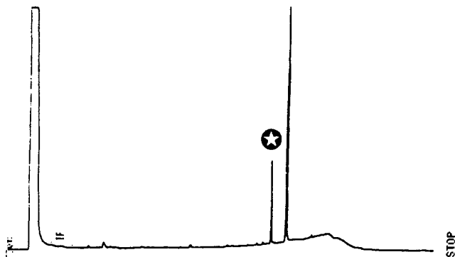
Figure 1. Gas chromatographic profile of a batch of N -phenyloleyleamide (NPOA) obtained according to method A. Separation was achieved on a glass capillary SE-30 column, as described in the text. The NPOA peak eluting at 16.96 min represents a 78.9% of the total integrator computed area under the peaks. The peak marked with the star, eluting at 16.08 min, represents 21.0% of the total area.
